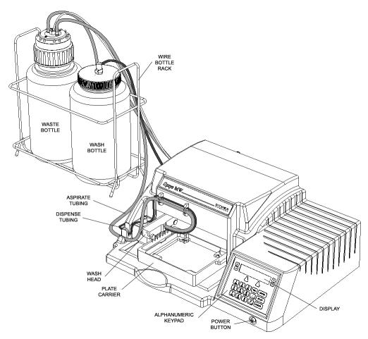
Figure 1. The Opsys MW™ Microplate Washing System
